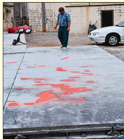
Figure 2. After 24 hours, a chain-drag survey revealed that 1.4% of the slab surface was delaminated (spray-painted areas). A worker marks the delaminated area with spray paint.
