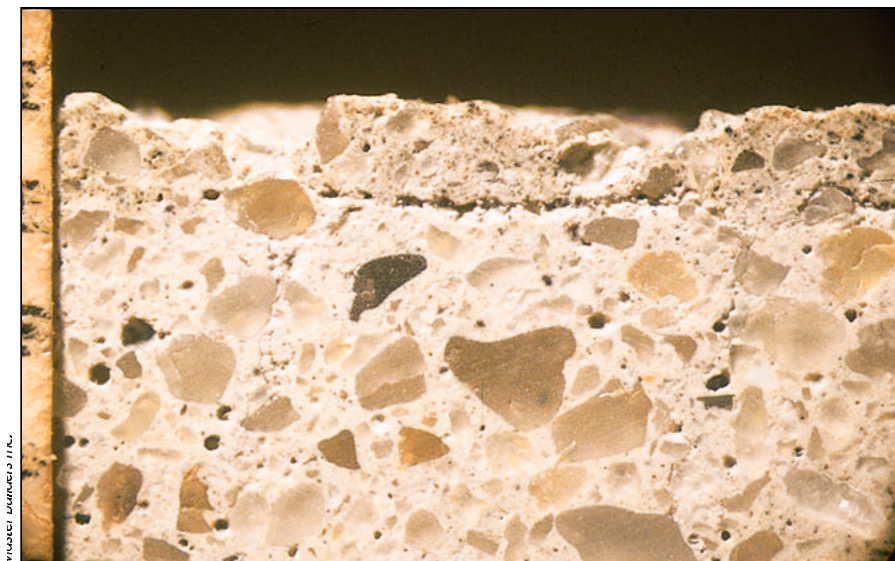
Figure 1. In this photomicrograph of an incipient delamination the connected elongated voids are 1 mm below and parallel to the finished surface. Each hatch mark on the left side of the slab is 1 mm.
