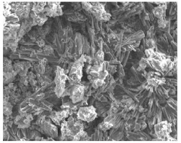
SEM micrograph of geo polymer concrete
