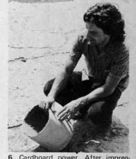
6. Cardboard power. After impregnation with sulphur this cardboard bucket became rigid enough to stand on. It held water without leaking for
